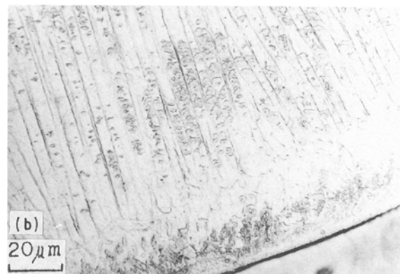
Figure 4 Stainless steel layer on mild steel by plasma arc cladding (Filler metal = 3.2 mm \phi Fe-23.3 wt % Cr-13.6 wt % Ni, arc current = 100A, travel speed = 2.67 mm s -1 , etchant = aqua-regia): (a) cellular austenite structure in the deposit region; (b) cellular dendritic austenite in the fusion boundary region; (c) austenitic matrix precipitating \sigma -phase in the fusion boundary region.
